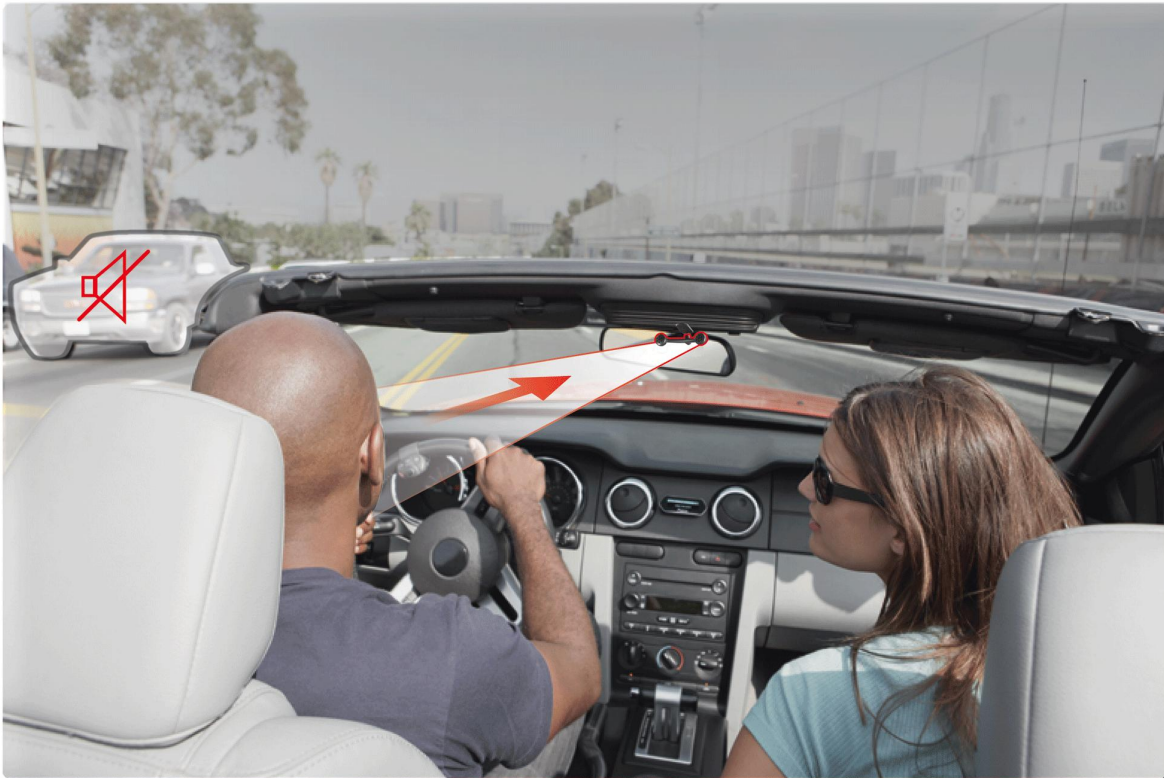
Lateral noise detection effect activated – Microphone correctly installed
