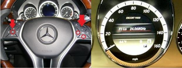
F1 Low: Set F1 Low by pressing 'OK' on the left side and 'Left' and 'Down' on the right side.
