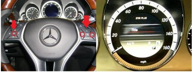
Reset: The interface can be reset to factory settings by pressing 'OK' on the left side and 'UP', 'DOWN','LEFT', 'RIGHT' on the right side. The factory settings are as follows:Title: ESCORT 9500F1 Low: 24.061F2 Low: 24.165F2 High 24.225
