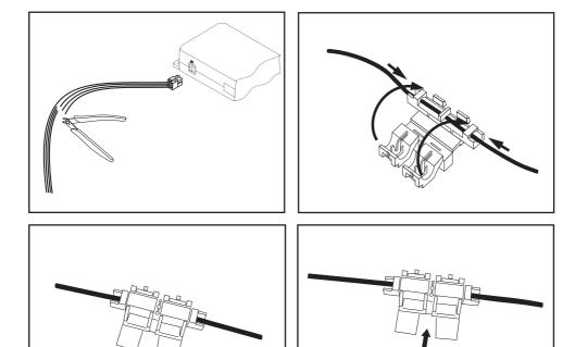
Please cut through the red, the black and the blue cable by means of a wire cutter or scissors. Now insert the two endings of the red cable resulting from the cut into one of the binders, then close it. If you hear two clicking noises, the clamp snapped in properly. Now insert one of the fuses and then repeat the procedure with the other cables.
