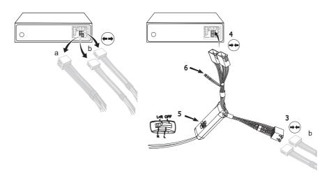
Depending on the switcher position (5), the voice of your conversation partner will be fed back through either the front right speaker, the front left speaker, or through both of the front loudspeakers. The 'OFF' position is to be selected if you connect the switchbox to the radio using the 'Phone-IN' cable (6).
